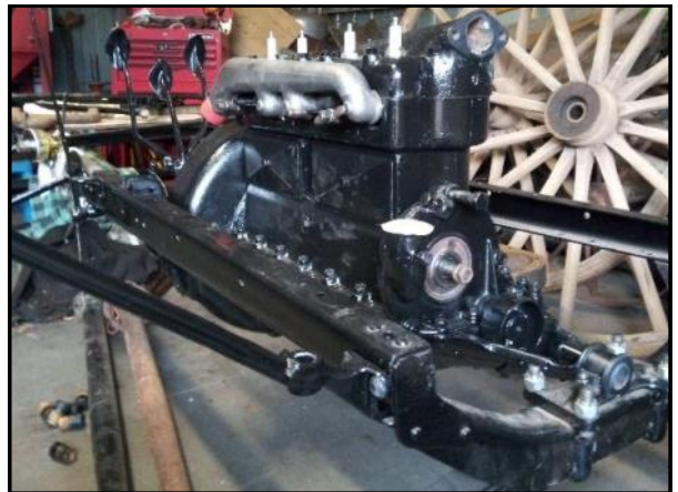
Newly rebuilt and restored engine, transmission and brass radiator mounted in the restored chassis.
