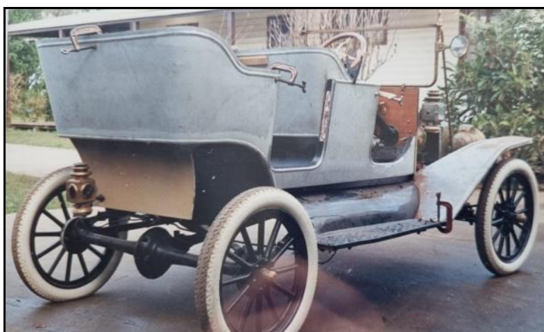
The second body fitted to Bill's 1912 was a new reproduction built to original Ford specifications in Bill's quest to get it all correct. Bill later replaced this body with a completely original body that he imported from one of his many trips to the USA.
