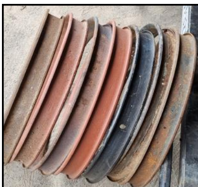
Original beaded edge rims ready for dimpling and lacing into the hubs
