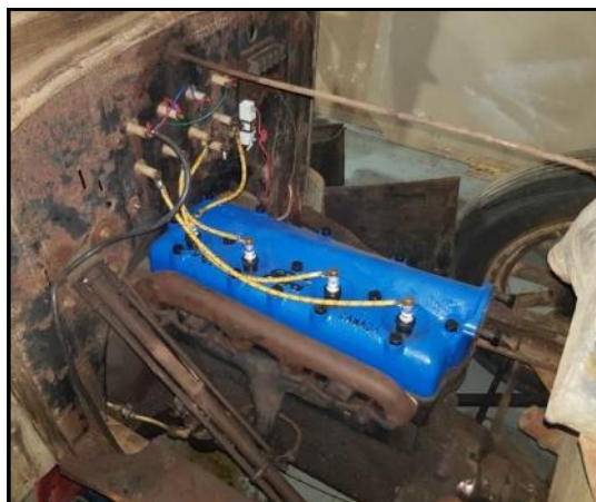
This TT is an early 26 Model. It features the 26 style steering column, and transmission cover but retains the earlier style 1925 Steel firewall and coil box mounting.
