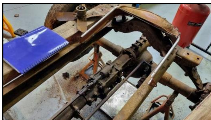
The TT rear axle featuring the inline auxiliary transmission.
