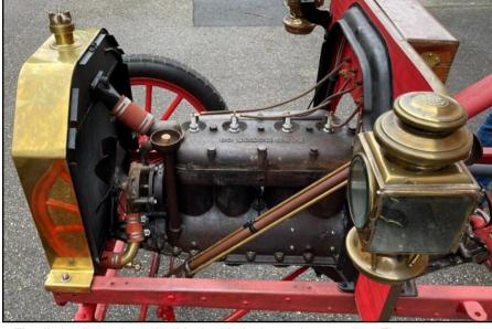
The distinctive 2 lever gear mechanism. The first 500 cars have become known as the '2 lever cars', as the second lever was used as a reverse in place of the pedal, which became a feature of all future production Ts. The reverse lever was a carryover from the previous Model N, R, & S models.
