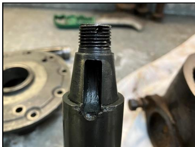
Damaged and loose driveshaft bearing sleeve.
