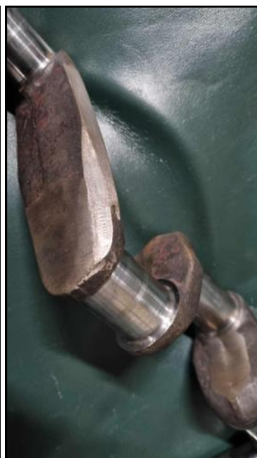
Large amounts of material ground away from the web.
