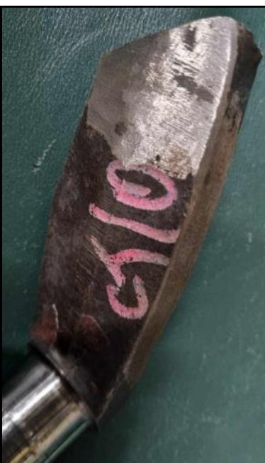
Material ground away all the way up to the bearing journal.
