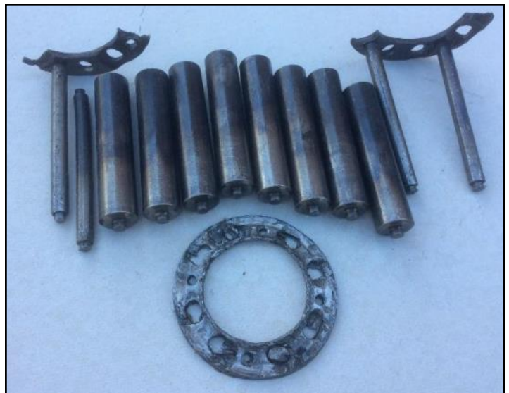
Destroyed pinion bearing hyatt roller bearing
