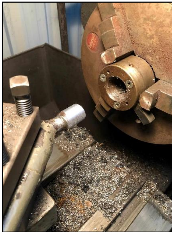
Worn ball built up and machined round in a special cutting jig.
