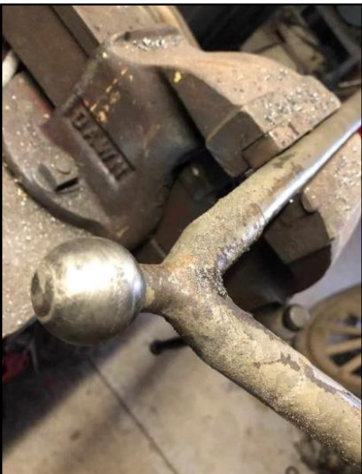
Finished round ball of a correct factory dimensions
