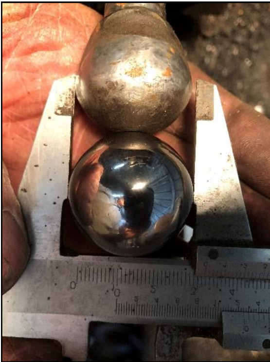
Proper spec ball and worn ball for comparison
